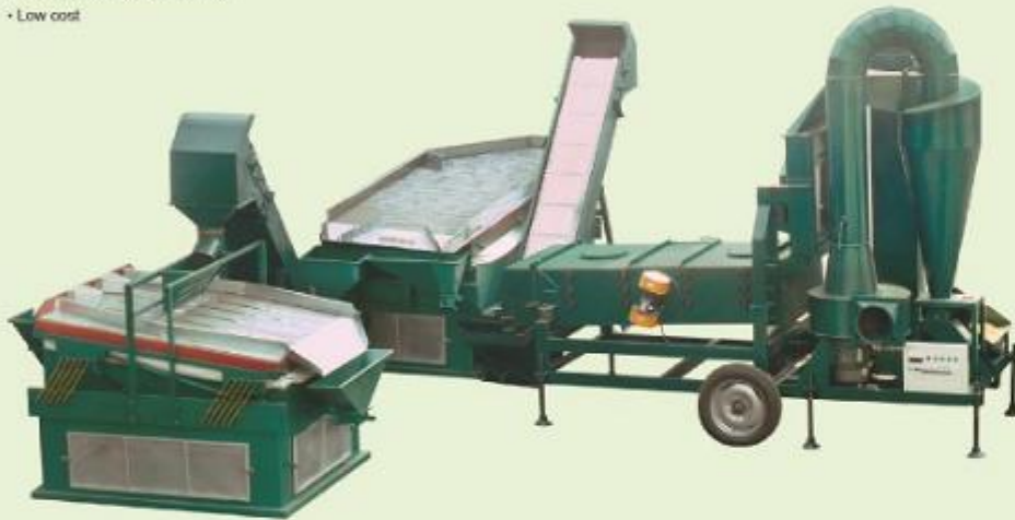
5XZC-5DH Seed Cleaner & Grader → 5XZ-5 Gravity Separator → 5XQS-5 Destoner
