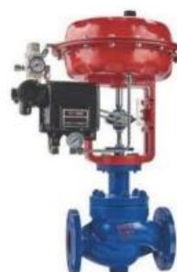
Multi-stage Decompression Type Control Valve Size : DN25-400 Pressure : PN16-64 Material : WCB/CF8/CF3M
